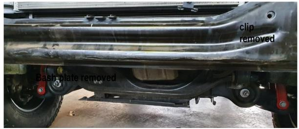
6) Now install the cradle centred with the 2 outer bolts on each side, you can use the 3 plastic tabs on the car infront of the radiator as centre link. The cradle is approx. 1100mm long & centre point is approx. 550mm
