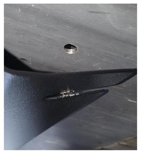
4) If your grill is moulded to the bumper you will need to air saw, Stanley knife or grind it away from the bumper, clean up and install in place with cable tie back to radiator support.
