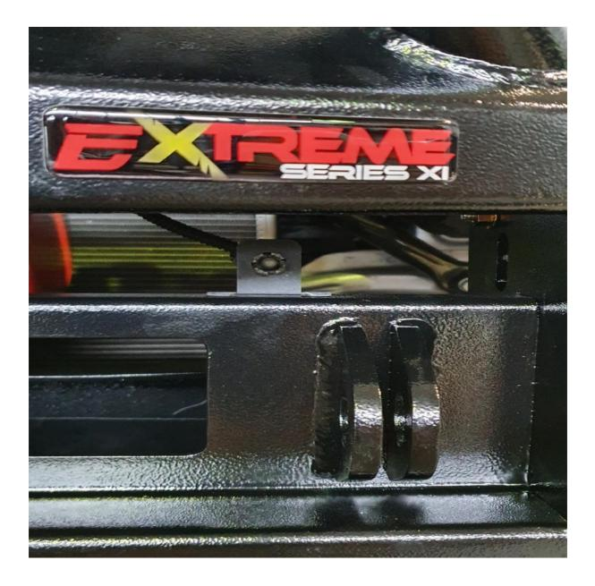
12) Cut the guards to suit profile of the bulbar and secure with cable tie to original metal support.
